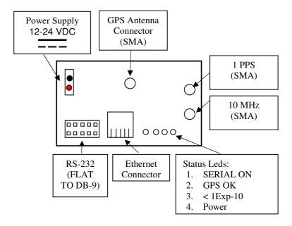
In order to power on the device a DC voltage 12-24V shall be applied on the power supply connector.
