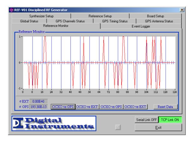
**NOTE:** These charts should never be confused with the internal systems used for the calculation of the internal oscillator disciplining. These graphs in fact allow a rapid evaluation of the system and any abnormal conditions that can occur mainly on the external back-up signal.
