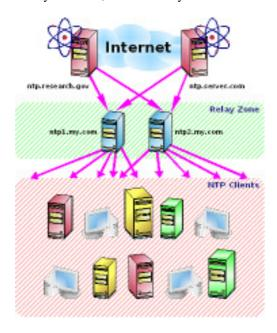
The device supports NTP server version 4 that distributes the synchronous time related to the GPS time reference.
